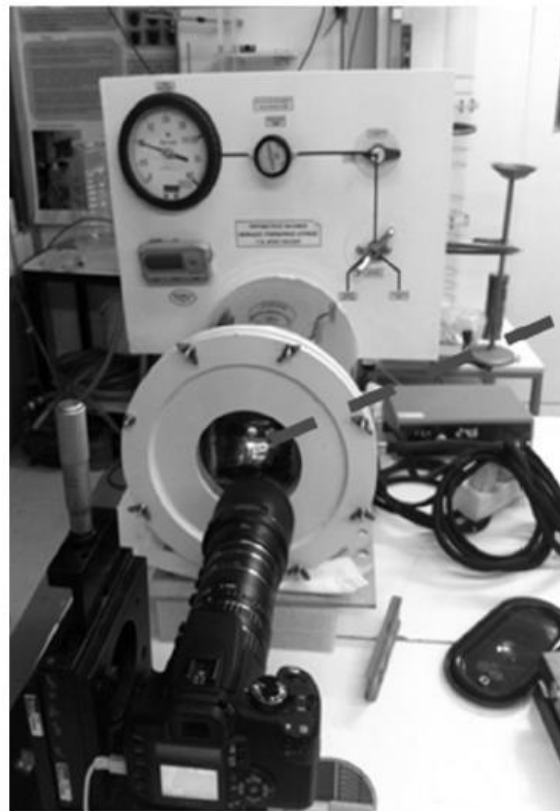
Fig. 2. Photograph showing the optical acquisition system and the temperature controlled small pressure chamber, as well as an example result.
